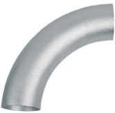
STBH Bend Elforsinket. Uten forlengede stusser. ø63–152 mm. 90°. T=2,9–4,5 mm. R= 157–380 mm.
